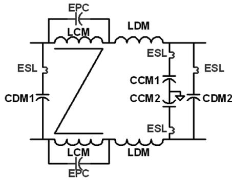
Fig. 1. Schematic of EMI filter.
