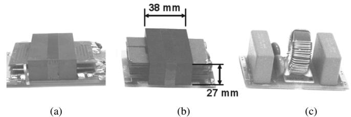
Fig. 16. Constructed prototypes: (a) improved integrated EMI filter, (b) previous integrated EMI filter, and (c) discrete EMI filter.
