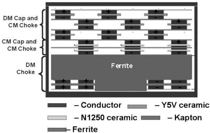
Fig. 7. Cross-sectional view of the half winding window of an integrated EMI filter structure.
