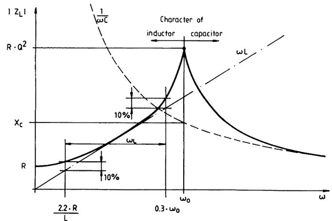
Fig. 4. Impedance versus frequency of a choke [8].
