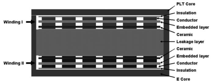
Fig. 15. Cross section view of half winding window of improved integrated EMI filter.
