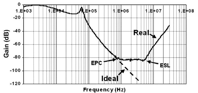
Fig. 5. Typical transfer gain of LP filter.
