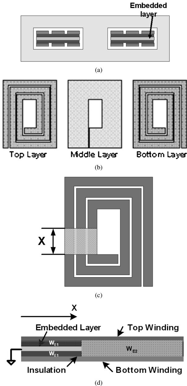
Fig. 10. (a) Planar winding w/embedded layer. (b) An example of winding and embedded layer layout. (c) Definition of design variable "X." (d) Side cross-section view of windings with embedded layer.
