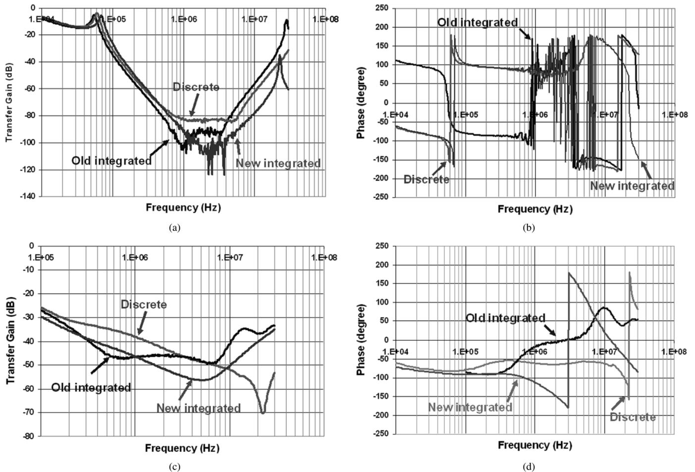
Fig. 17. (a) DM transfer functions: gain. (b) DM transfer functions: phase. (c) CM transfer functions: gain. (d) CM transfer functions: phase.
