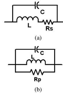
Fig. 3. (a) Equivalent circuit 1 of a choke. (b) Equivalent circuit 2 of a choke.
