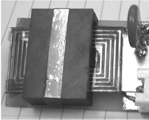
Fig. 13. Low-pass filter with planar inductor.
