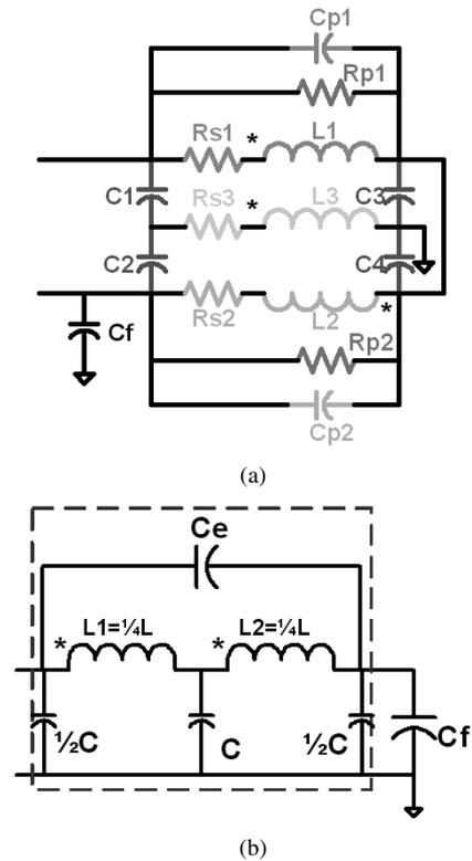
Fig. 11. (a) Equivalent circuit of planar inductor w/embedded layer. (b) Simplified equivalent circuit.
