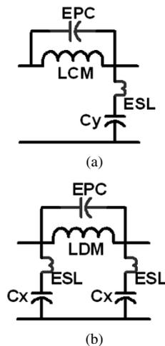
Fig. 2. (a) Equivalent circuit of CM filter. (b) Equivalent circuit of DM filter.
