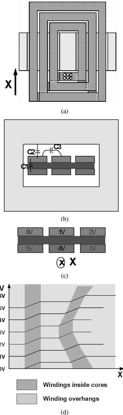
Fig. 9. (a) Top view of cross section of a planar spiral winding. (b) Front view of cross section of half winding window. (c) Voltage distribution of cross section—front view. (d) Voltage distribution along winding length.
