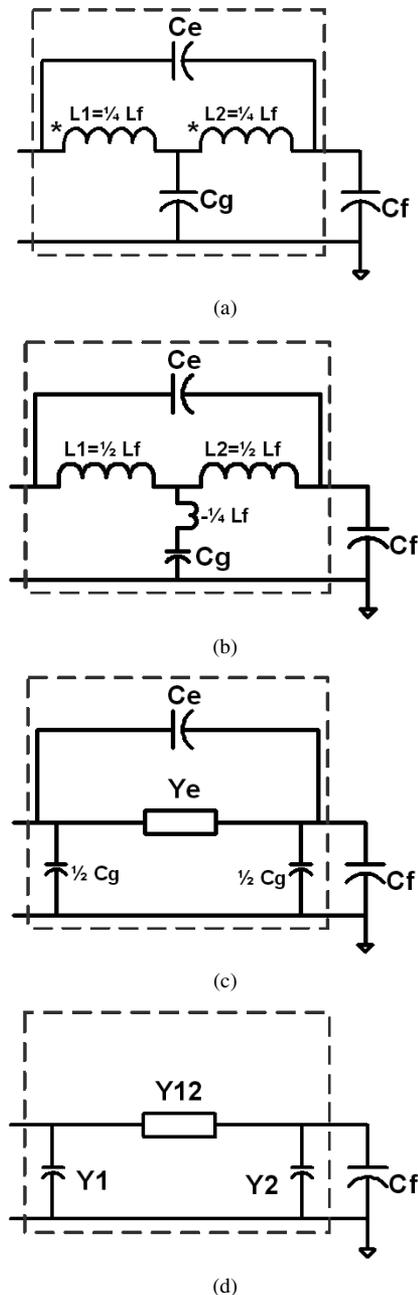
Fig. 8. (a) Schematic of inductor w/parasitic capacitance canceling. (b) Decoupled equivalent circuit. (c)  $Y/\Delta$  transformation results. (d)  $\pi$  equivalent circuit.
